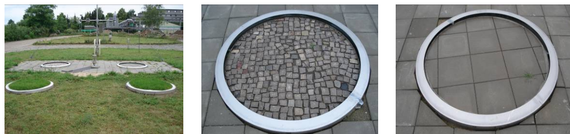
Figure 3. Views of lysimeter with cobble stones and concrete plates.
